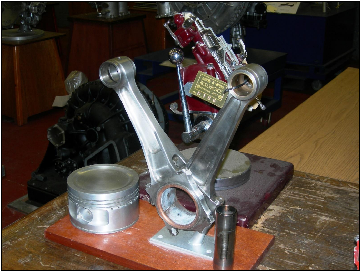
Forked conrods and a piston and gudgeon pin from a Merlin engine.
