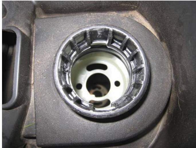
Scooter petrol tank showing overflow guard
